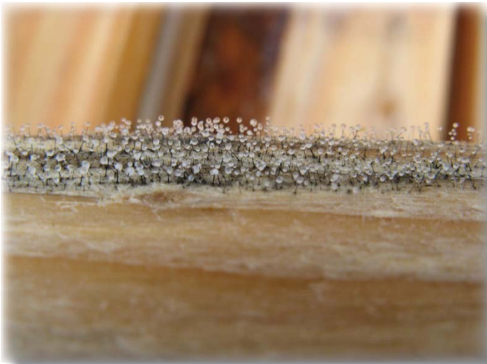
Stain conidiophores on wood surface may look like mold – dark hyphae and wood below indicate stain.
