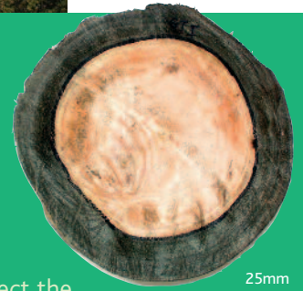
25mm full sapwood TANALITH preservative penetration on eucalyptus pole, ensuring a long term and permanent protection.
