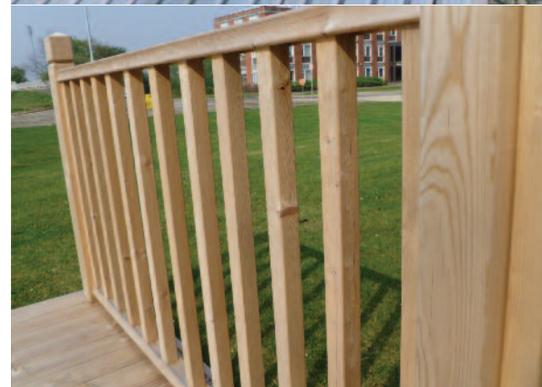
Field tests used to assess the aesthetic and protection performance of cladding and decking timbers
