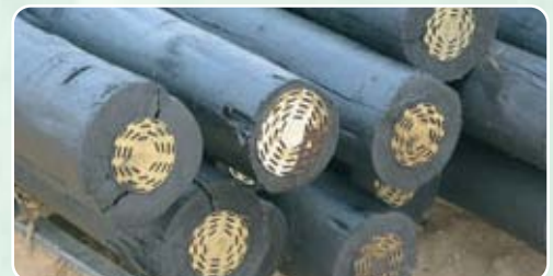
Creosote can leach from treated timber and taint the surrounding environment.
